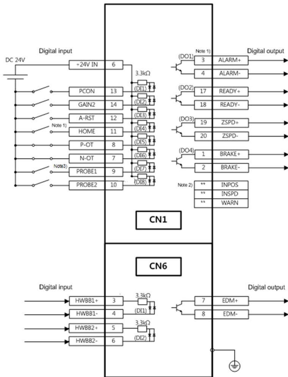
Note 1) The input signals (DI4~DI8, output signals (DO1~DO4) are the factory default signals.
