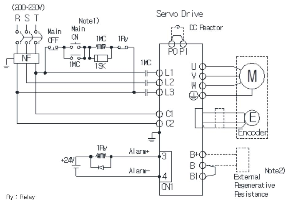
**Note 1)** It takes approximately one to two seconds to output an alarm signal after turning on the main power.
