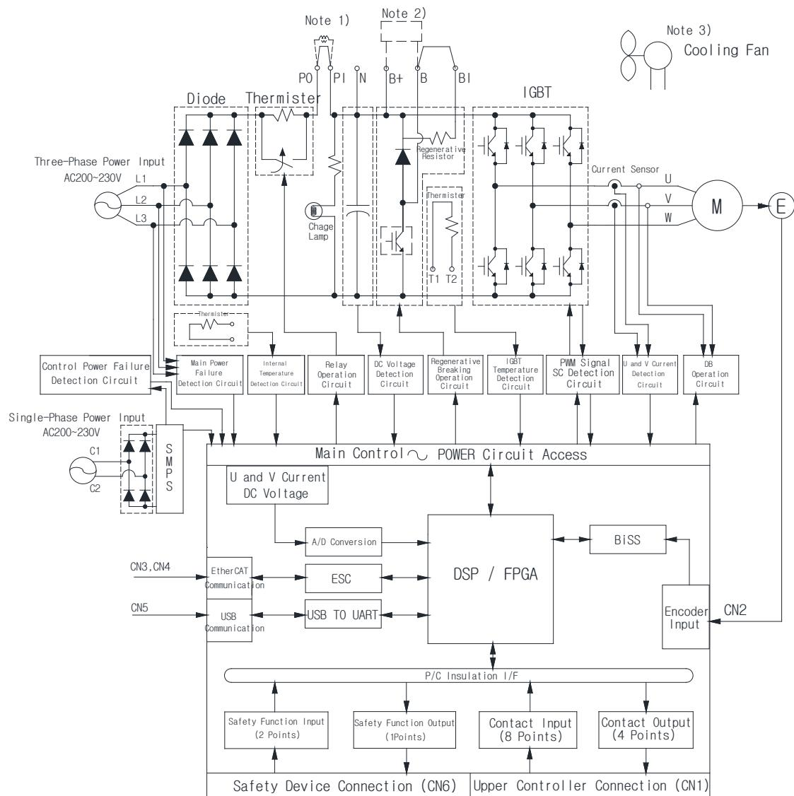
**Note 1)** If using a DC reactor, connect the PO and PI pins.
