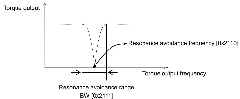
Mechanical resonance causes vibrations to occur at certain frequencies in certain systems. You can control the vibrations by controlling the torque output for specific frequencies.
