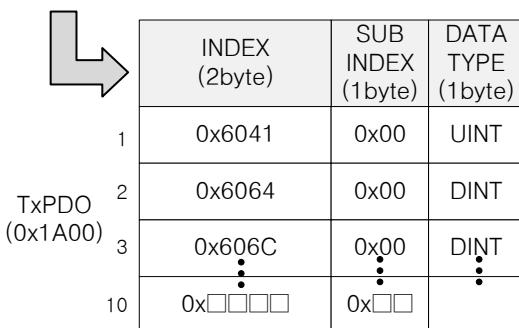
The SyncManager can be composed of multiple PDOs. SyncManager PDO Assign Object (RxPDO:0x1C12, TxPDO:0x1C13) indicates the relationship between the SyncManager and the PDO.
