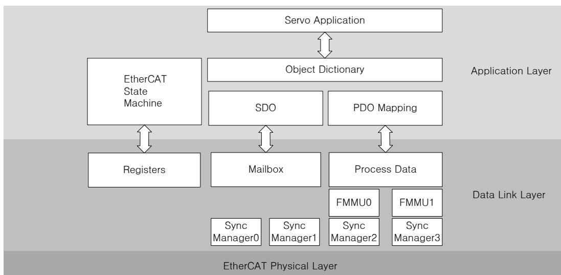
The XDL-L7N drive uses a CiA 402 drive profile. The Object Dictionary in the application layer includes application data and PDO mapping information from the process data interface and application data.
