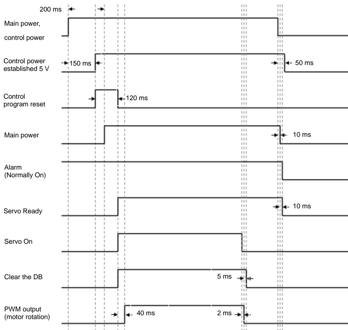
**Note 1)** The Servo Ready turns on after the main power is established and the control program is reset.
