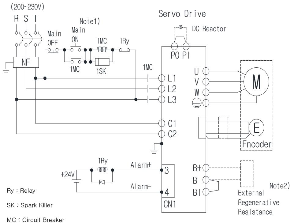
It takes approximately one to two seconds to output an alarm signal after turning on the main power. Accordingly, press and hold the main power ON switch for at least two seconds.
