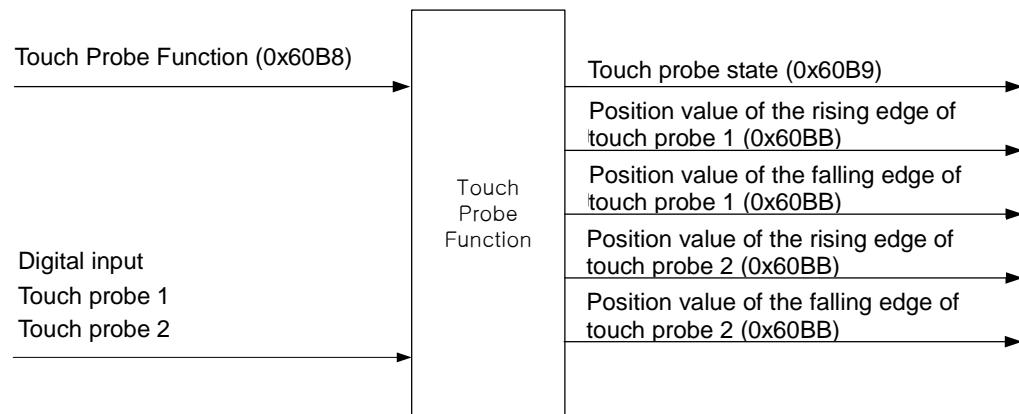
Position feedback is latched to the following trigger events:
