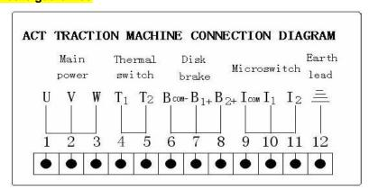
Always connect the frequency inverter output and earthing terminal to motor terminal as shown in the picture. The connection cable diameter is decided accordingly to the motor rated current (can refer to frequency inverter instruction manual).
