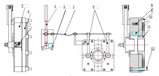
Working Stroke Gap  $\leq$  0.4 mm
