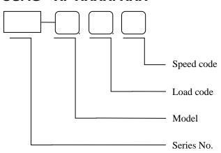
For example: CSAG-L.1000.100 Type means this machine is CSAG-L gearless PMS elevator traction machine, rated load is 1000kg, and rated speed is 1.0m/s.
